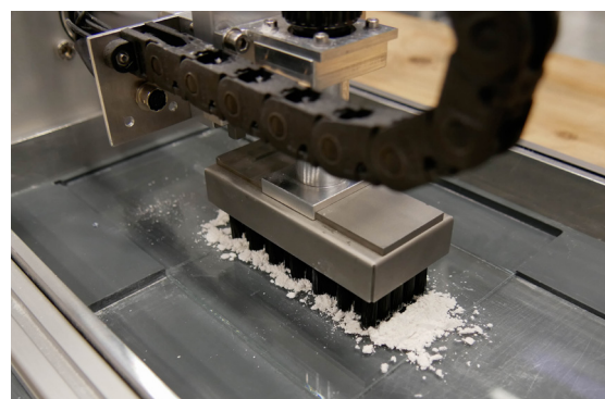
Abrasion test with linear brush cleaning under the influence of a standardized test dust.
